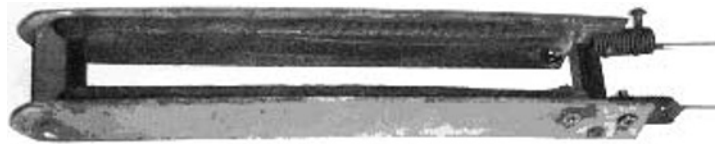
Fig. 3. Appearance of an electrolysis cell made of the C-C material.
